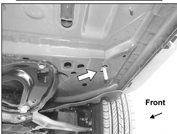
(Fig 14) Insert "Long" Bolt Plate into oval hole in front floor location (arrow)
