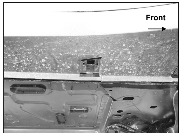
(Fig 2) Passenger/right #2 clip removed
