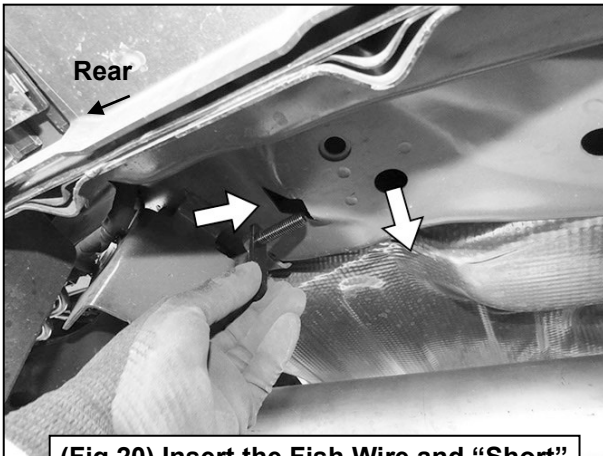
(Fig 20) Insert the Fish Wire and "Short" Bolt Plate assembly into square hole and down through floor (arrow)
