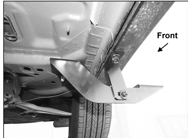
(Fig 16) Passenger/right front Mounting Brackets installed
